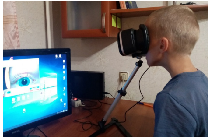
Figure 1. Appearance of the computer appliance hardware for objective determination of the eye movement range
