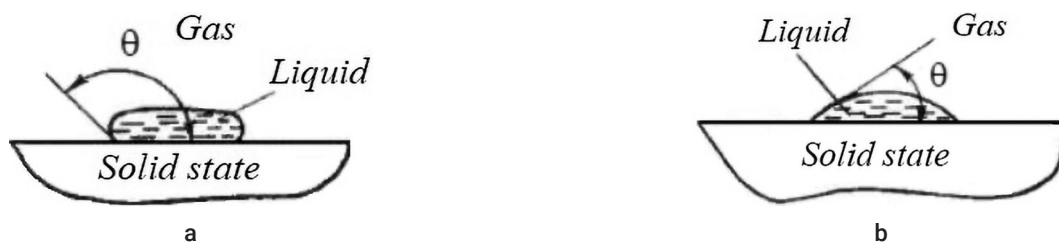
Figure 10. Schematic representation of the liquid droplet shape and the wettability angle at the membrane solid horizontal surface: a – \theta exceeds 90^\circ – the surface wettability is low; b – \theta is less than 90^\circ – the surface wettability is high
