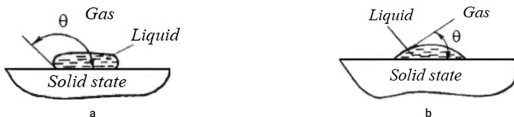
Figure 10. Schematic representation of the liquid droplet shape and the wettability angle at the membrane solid horizontal surface: a – \theta exceeds 90^\circ – the surface wettability is low; b – \theta is less than 90^\circ – the surface wettability is high
